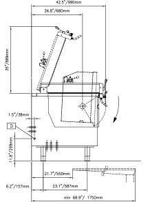
CWII = Cold Water inlet 1 (cleaning) Electrical inlet (power) ΕI Hot water inlet
